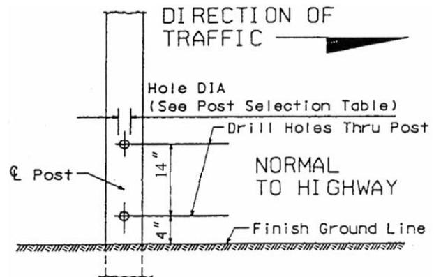
**Note:** Posts that are larger than 6 x 8 require barrier protection when located within the Control Zone.
