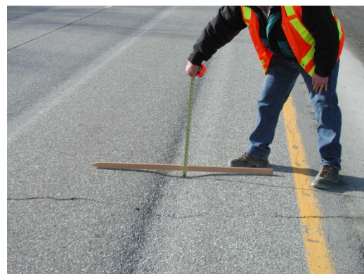
Figure A3.2. Studded Tire Wear on HMA
