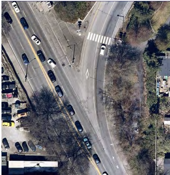
Before: aerial of ramp with two full-time lanes, a general-purpose lane, and an HOV bypass
